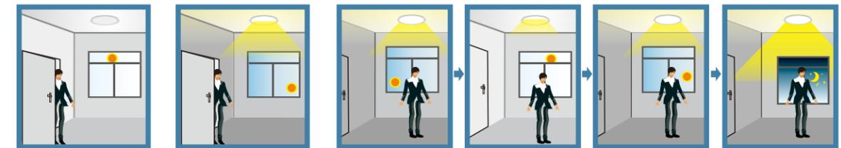
When the ambient light is larger than the present illumination level (Set by 1-10V daylight sensor), the lamp stays off.
