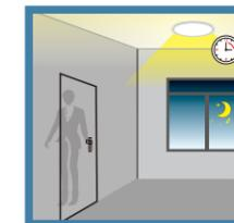
If there is insufficient ambient light, the lamp dims to a stand-by dimming level (Set in the motion sensor) when no motion is detected during hold time, it will switch off after stand-by period.
